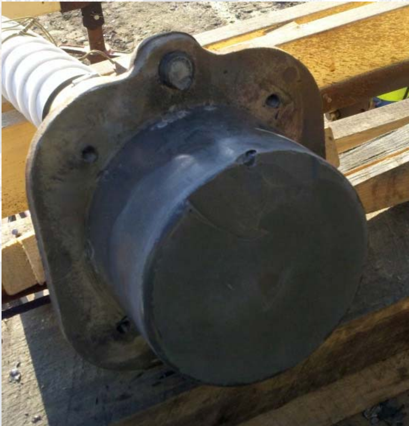
Grout 3 no void or soft grout
