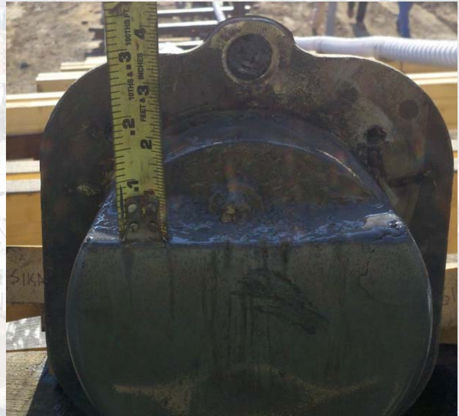
Grout 2 void and soft grout
